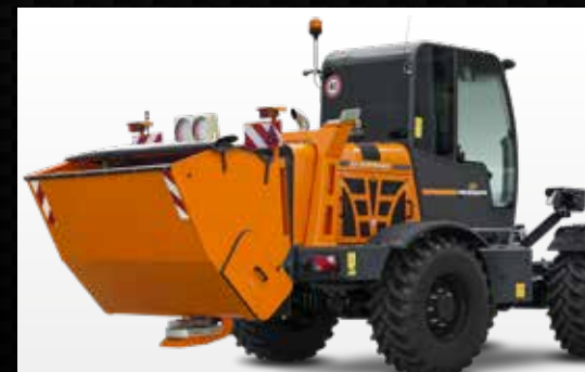
SPARGISALE AUTOCARICANTE SELF LOADING SALT SPREADER
